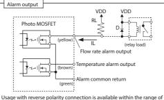
rated voltage and current as shown below, by specifying the alarm mmon return specification when placing an order. (connecting RL, VDD to the common return) Use with VDD < 40 V, I < 100 mA (Example: VDD = 24 V, RL = 5.1 k $\Omega$ )
