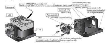
For the single unit fitting block, it is possible to fix its bottom (by using two M4 hexagon socket head cap bolts), to fix its rear (by using two M4 countersunk head screws), or to fix with a pipe, depending on the mounting dimensions
