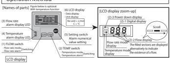
Turning ON the DC power, (2)-1 displays flow rate in digital, and simultaneously (2)-2 scrolls from left to right to ndicates the existence of a flow. It scrolls at a constant speed regardless of the flow rate (No scroll indicates no flow)
