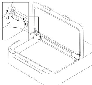
2. Remove springs from the frame and insert the lid into the frame
