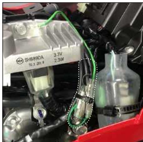
Connect Black wire of ①Tachometer to ②Power wire and Green wire to ③GND wire. Connect Black/White of ①Tachometer to ④IG coil branch wire.
