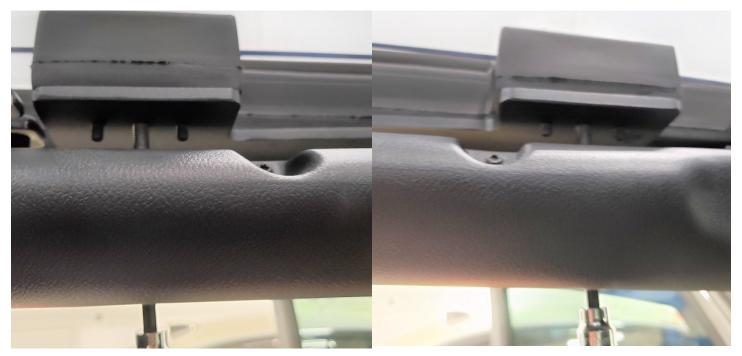
6. Tighten the M8 bolts leaving a small gap between the Skyview hardware and the roll bar on the vehicle. Do not overtighten.
