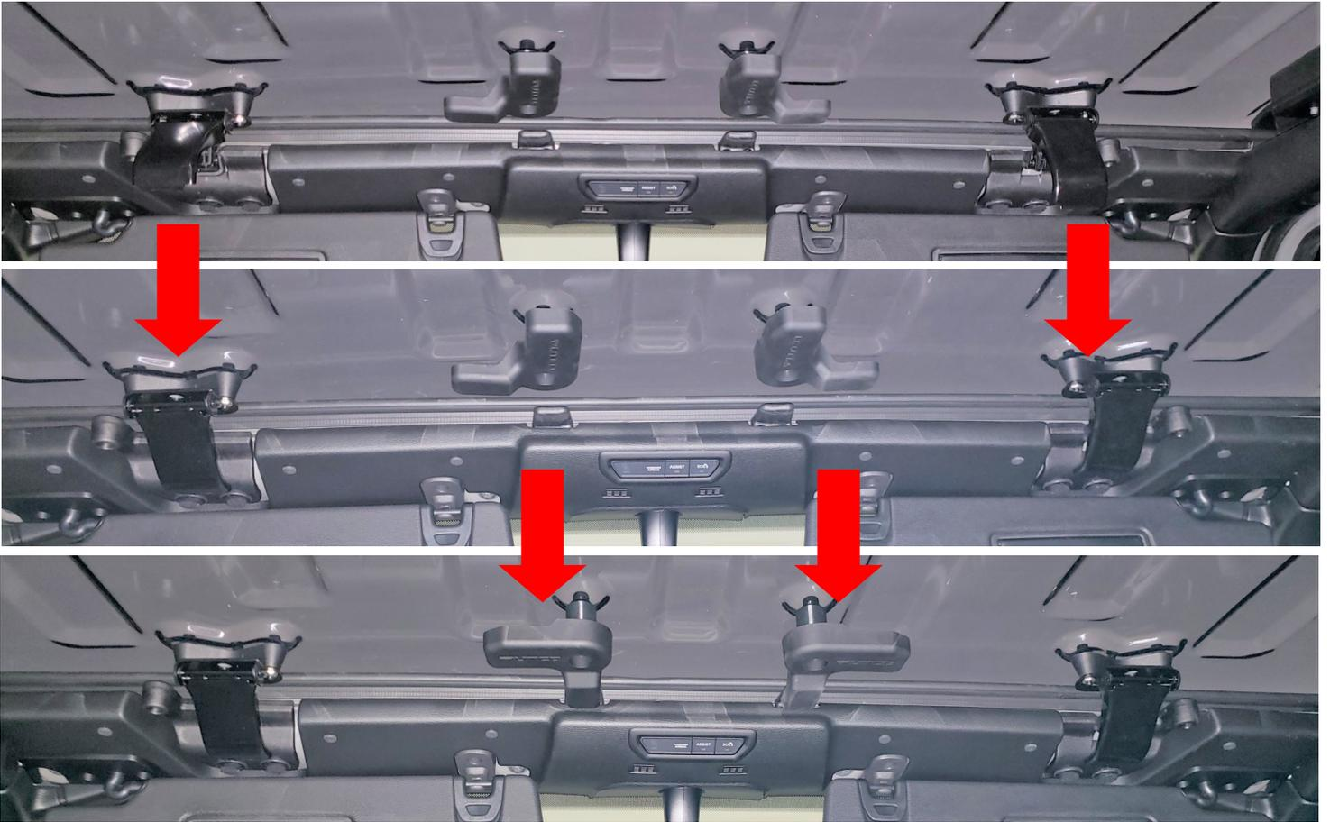
4. Close the rear two L-shaped clamps. (picture pointing to the rear clamps)
