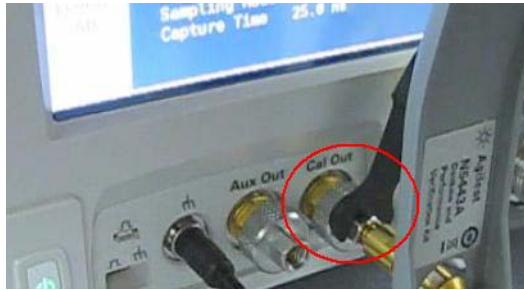
Figure 73 Tighten to 8 in. lbs.
