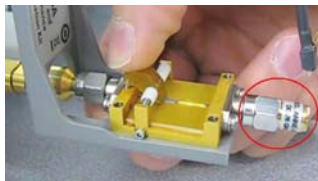
Figure 71 50Ω Terminator on N5443A
