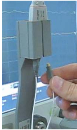
Figure 76 Connect the Head to the Probe
