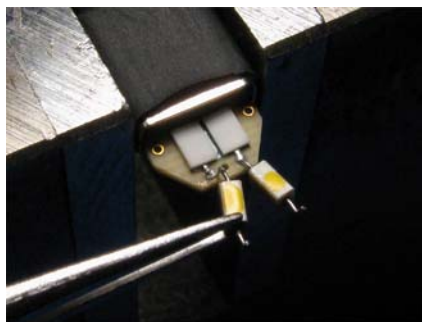
Figure 62 Soldering in a new axial resistor
