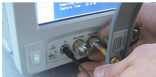
Figure 72 Attaching the N5443A Fixture
