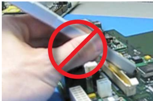
Figure 38 Improper Probe Handling
