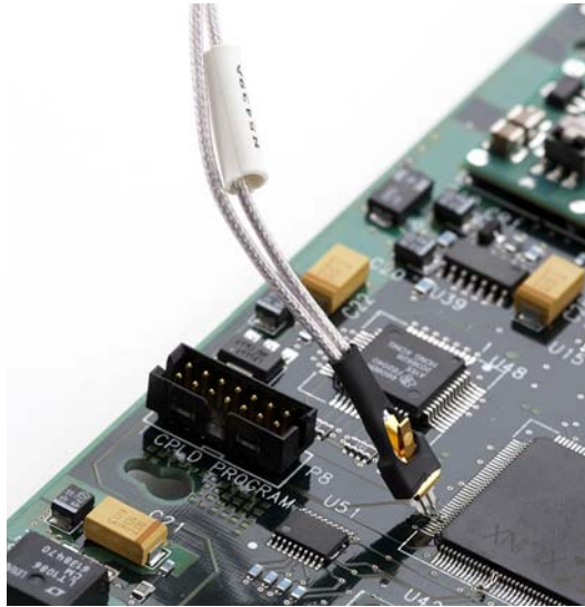
Figure 31 Probe Oriented Perpendicular to Device
