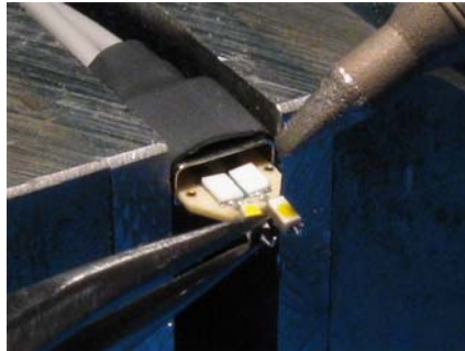
Figure 60 Removing the Resistor
