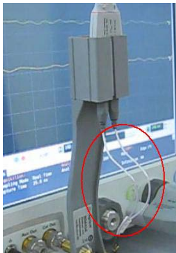
Figure 77 Positioning the Probe Head Wires
