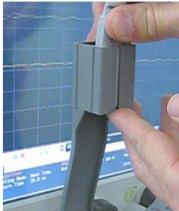
Figure 74 Inserting the Probe Head
