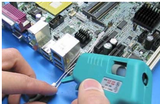
Figure 57 Probe Secured Using Low-Temperature Hot Glue
