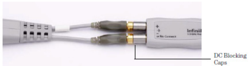
Figure 17 Blocking Caps Between Probe Amplifier and Head
