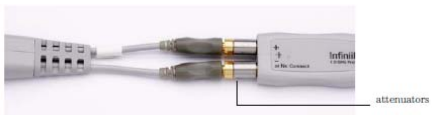
Figure 13 Placement of Attenuators Between Probe Amplifier and Head
