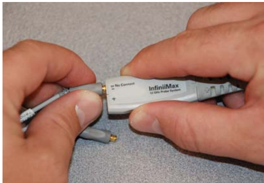
Figure 4 Properly Pulling the Probe Head Straight Out
