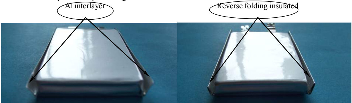
Fig.2. Single folding edge schematic of PL cells
