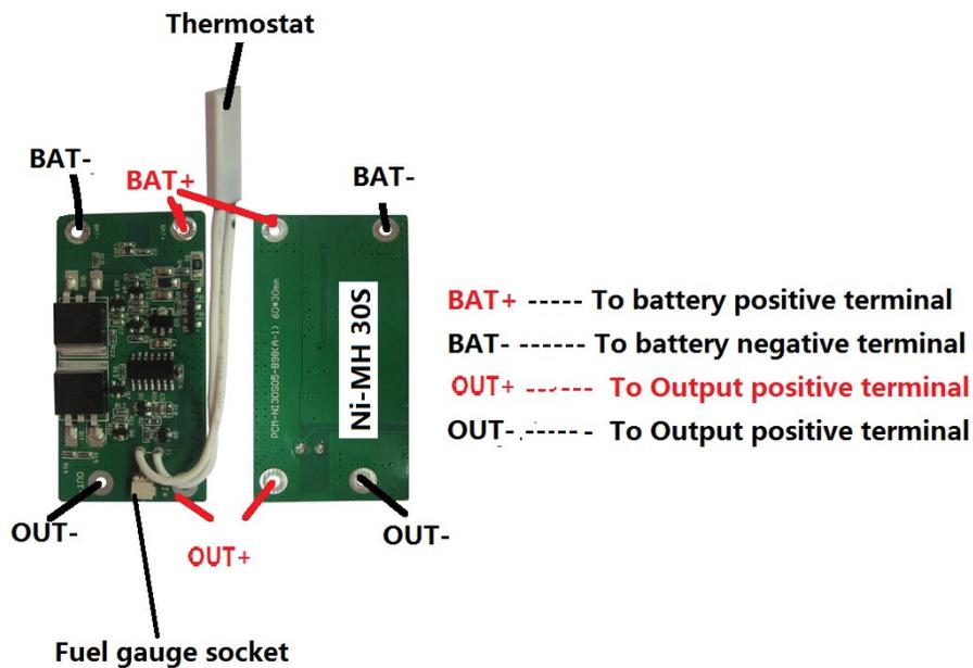
3.3 If you want to install a fuel gauge to monitor the battery's voltage, connect our fuel gauge (Part No: [FG-MH30S](#)) in fuel gauge socket, as shown below.
