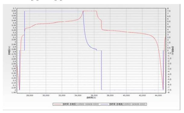
40152SE discharging and charging curves at discharging rate of 1C:
